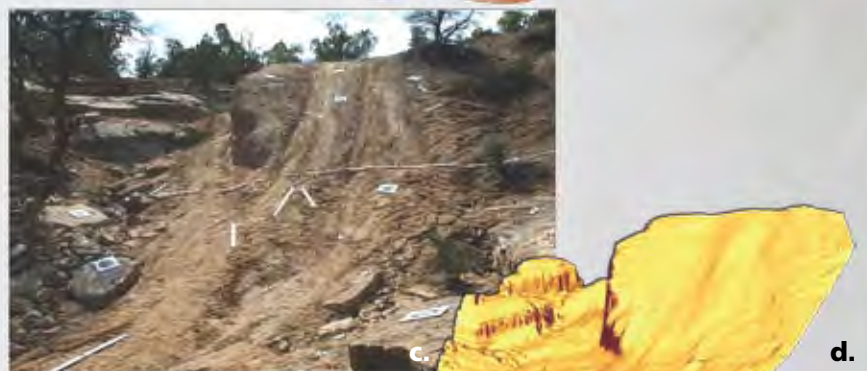
c. Photograph taken in September 2006. d. 3D surface model generated from the 2006 photography rendered as a hillshade (Ypsilantis et al. 2007).
